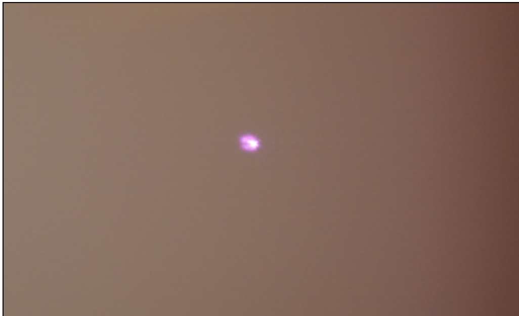
Figure 67: Spot Size using Plano-Convex Cylindrical Lenses and Thorlabs L904P010 905 nm Near Infrared Laser Diode (No Permission Needed)
